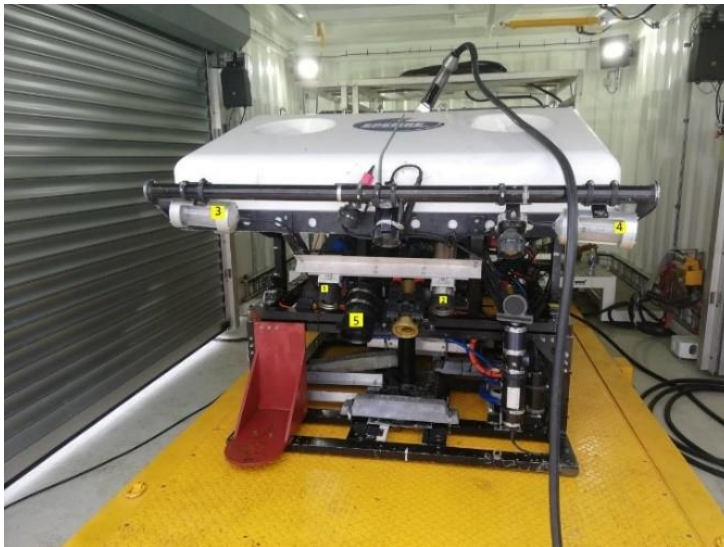
Figure 14: The Sperre SUB-Fighter 30K. (1) and (2): Avt GC1380C cameras. (3) and (4): Lights. (5): videocamera. Picture: Benjamin Morris King
