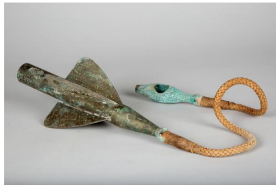
Figure 26: A chip log located at the stern of the ship. Used for measuring speed known as knots. The picture on the left from https://www.digitaltmuseum.no .
