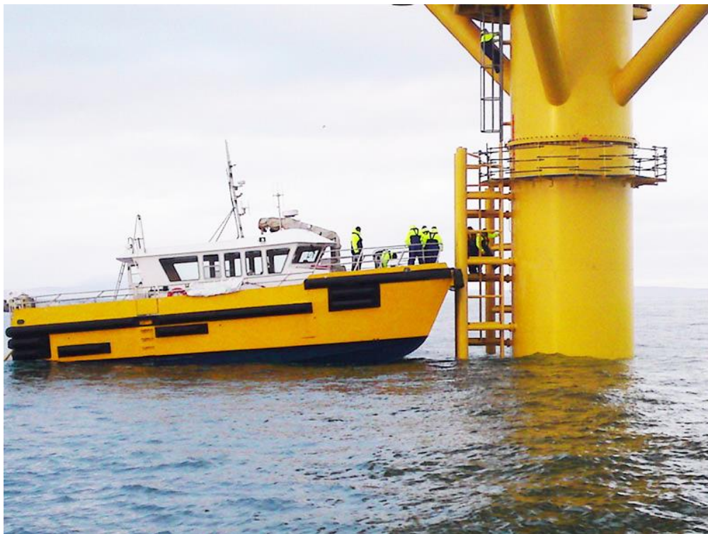
151 Fig. 4 Fender docking operation of the maintenance ship against wind tower.
