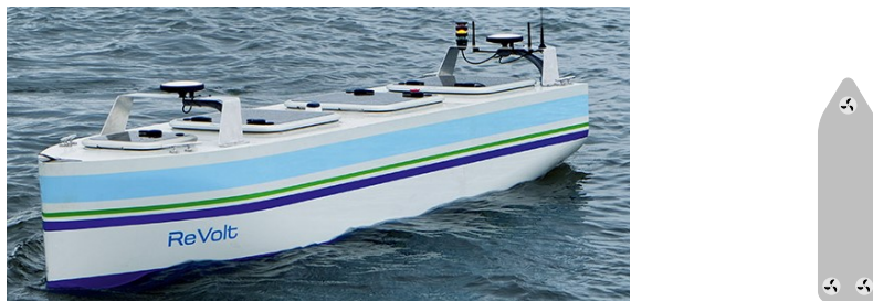
Figure 2: The ReVolt test platform is a 1 : 20 scale model of a autonomous concept vessel with two fully rotatable azimuth thrusters in the stern and one fully rotatable azimuth thruster in the bow.
