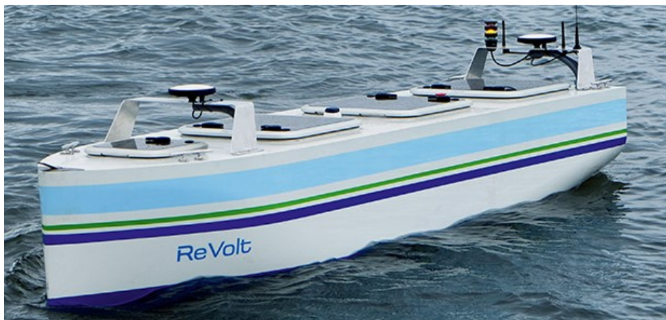
Figure 1.1: The ReVolt , a 1 : 20 scale model autonomous cargo concept vessel developed by DNV (then DNV GL).
