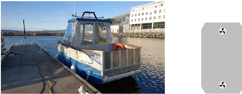
Figure 3: The MilliAmpere test platform has two fully rotatable azimuth thrusters along the centerline of the vessel.
