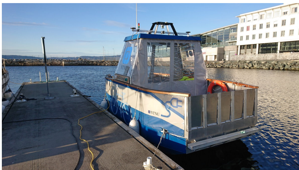
Figure 1.2: The milliAmpere , an experimental autonomous urban passenger ferry developed by NTNU.
