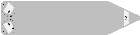
Figure 2: Thruster configuration for vessel, where 1 and 2 are azimuth thrusters, and 3 is a tunnel thruster.
