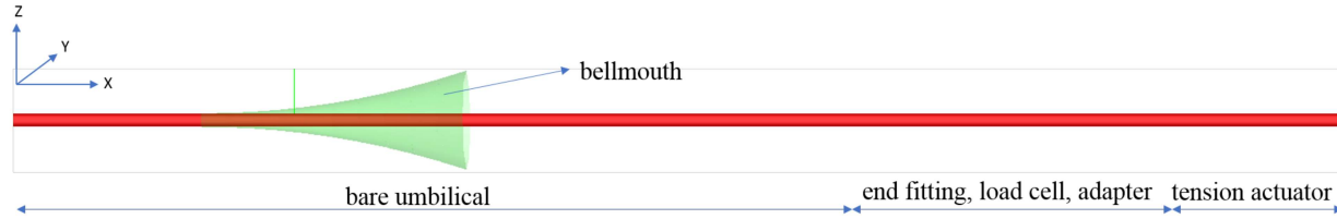
(a) Global model of full scale testing in BFLEX
