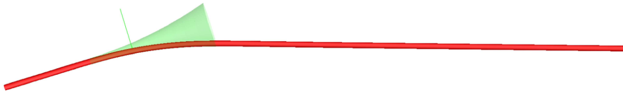
(c) The umbilical has full contact with lower surface of bellmouth
