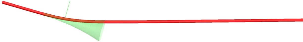
(b) The umbilical has full contact with upper surface of bellmouth
