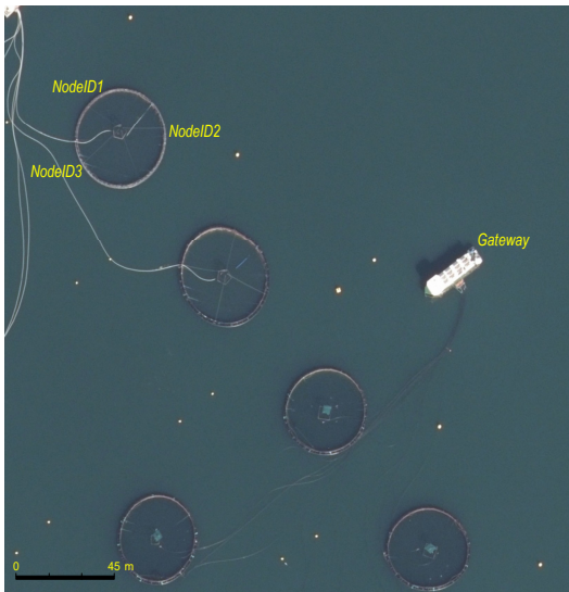
Fig. 5 Map showing position of nodes and gateway in the fish farm
