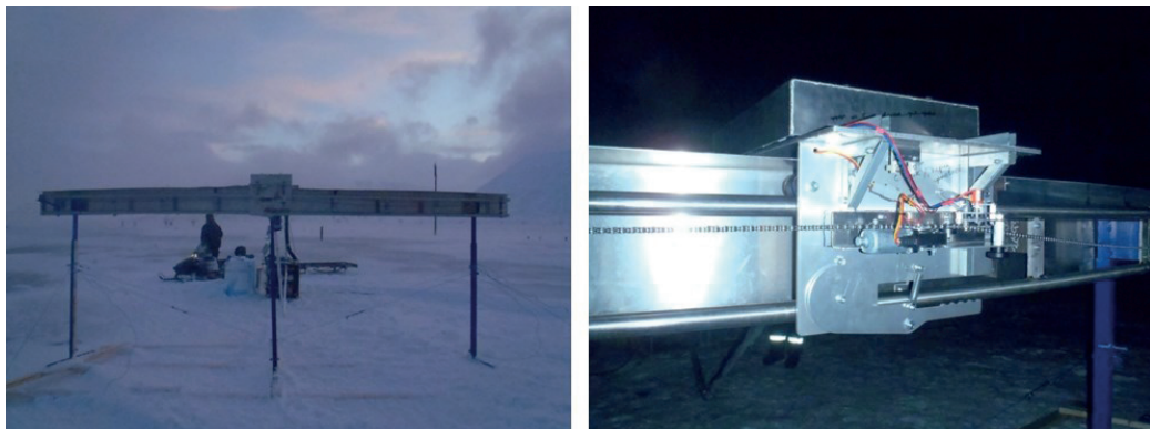
Figure 30. Pictures of the rail and the carriage from the back. Picture to the right shows the chain and motor which are used to move the target.
