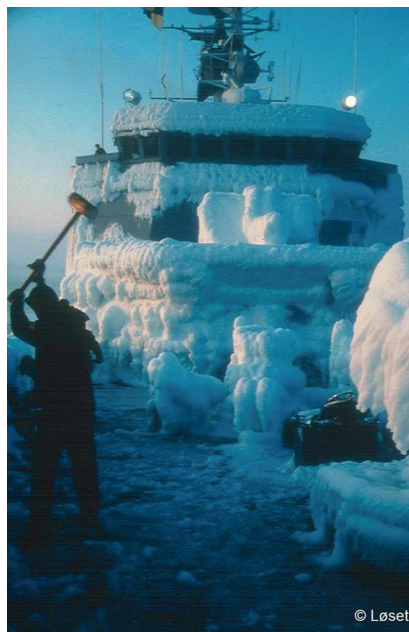
Figure 2. Icing on the K/V Nordkapp on the 27 th of February 1987. More than 110 tons of ice accreted in 17 hrs in storm conditions at an air temperature of -15^{\circ}\text{C} . Ice on the bridge window was already removed. Photo by Prof. Sveinung Løset.
