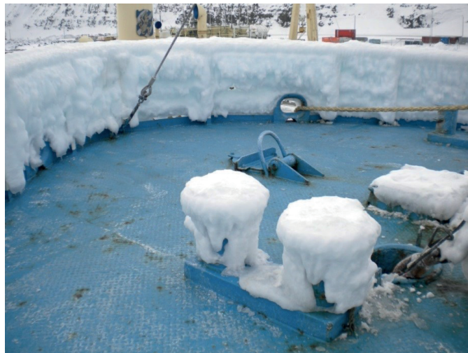
Figure 4. Ice accretion on the bow of the R/V Lance in May 2009. Photo by Prof. Sveinung Løset.
