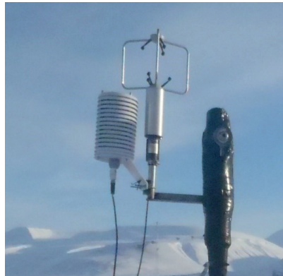
Figure 28. Weather station installed on the top of the spraying rig.
