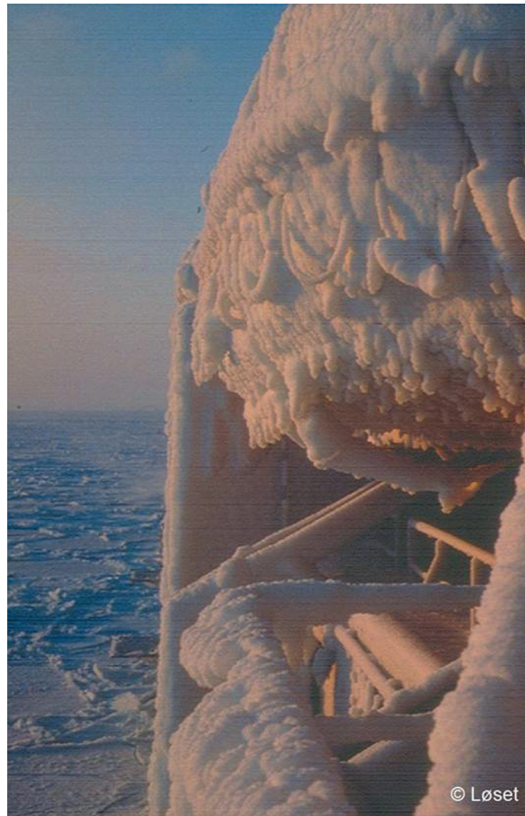
Fig. 1. The ice accreted on the starboard side of the Coast Guard vessel Nordkapp on 27.02.1987 while the vessel was moving against the waves.
