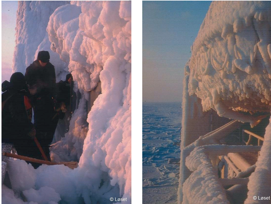
Figure 3. Icing on the starboard side (left) and on the rescue boats (right) of the K/V Nordkapp on the 27 th of February 1987. Photos by Prof. Sveinung Løset.
