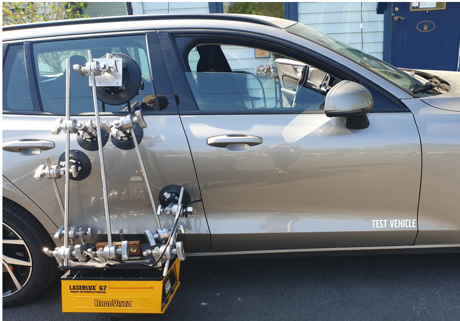
FIGURE 3.2: Retroreflectometer mounted on the side of the test vehicle.
