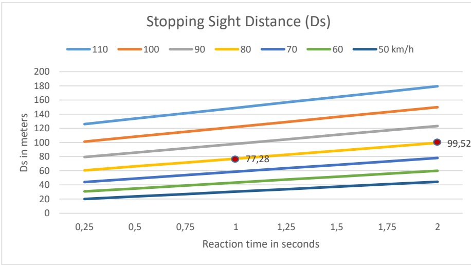
Figure 3 The effect of reductions in reaction time ( t_r ) and increases in design speed ( V ) on stopping sight distances
