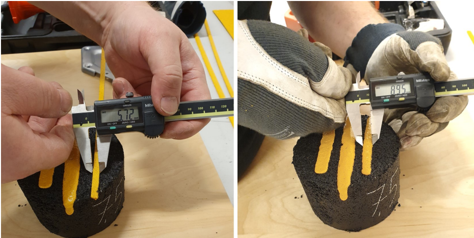
FIGURE 3.4: Difference in width of thermoplastic marking before (left-hand side) and after (right-hand side) melting.
