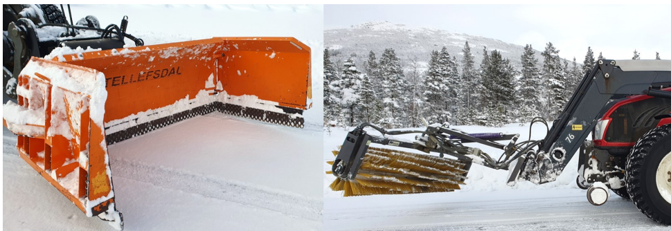
FIGURE 3.6: Snow removal equipment. Ribbed plow on the left-hand side and brush on the right-hand side.
