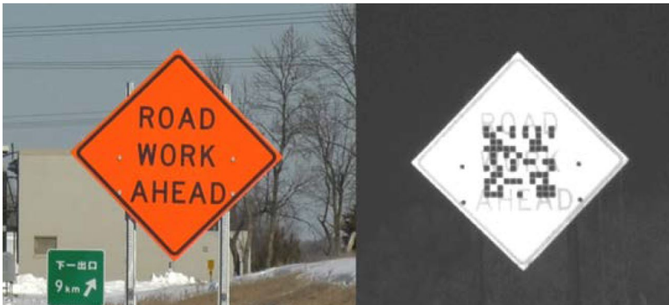
FIGURE 4.5: Sign with traditional layer and an added layer visible in the near infrared. Source: Snyder et al. (2018).
