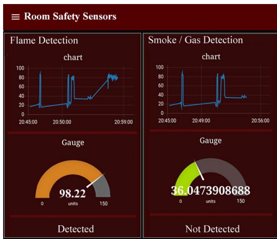
Figure 8. Dashboard of safety sensors in terms of graphs and gauges that are used for real-time monitoring to protect the property and human life from harm or damage.
