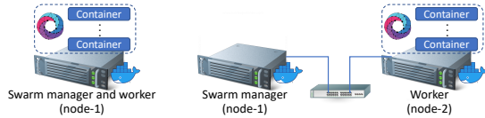
Fig. 3. Illustration of Manager (left) and Manager-Worker (right) deployment configurations and experimental testbed.
