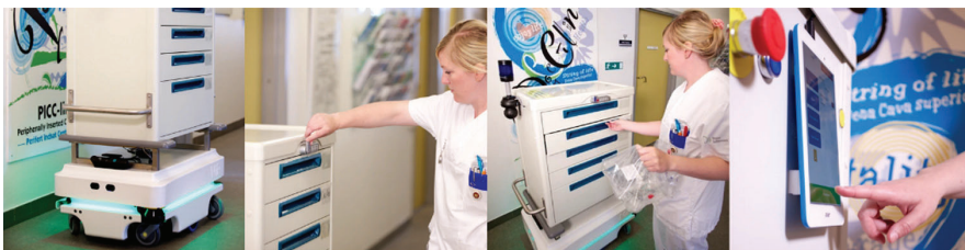
Fig. 2. Sending and delivery of cancer medicine with secured transportation [10]
