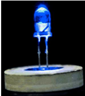
FIGURE 1.1. BLUE LED based on the GaN semiconductor material system 2,3 (adapted with permission from ref. 2 © 2015 John Wiley and Sons).
