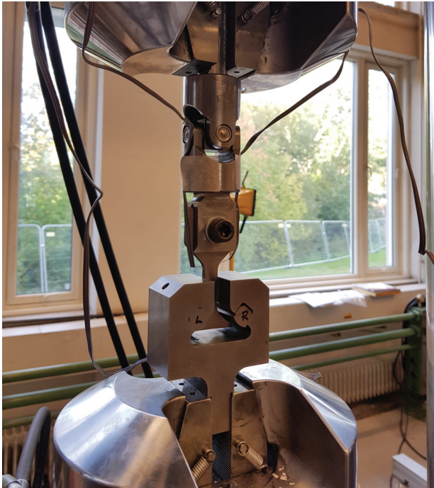
Figure 3.4: Titanium specimen with strain gauges attached to both flanks on the dovetail specimen
