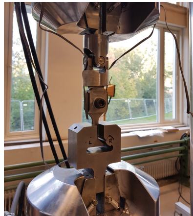
Fig. 3. Fixture mounted in multiaxial fatigue machine with a single Ti-6Al-4V specimen instrumented with strain gauges on both flanks.
