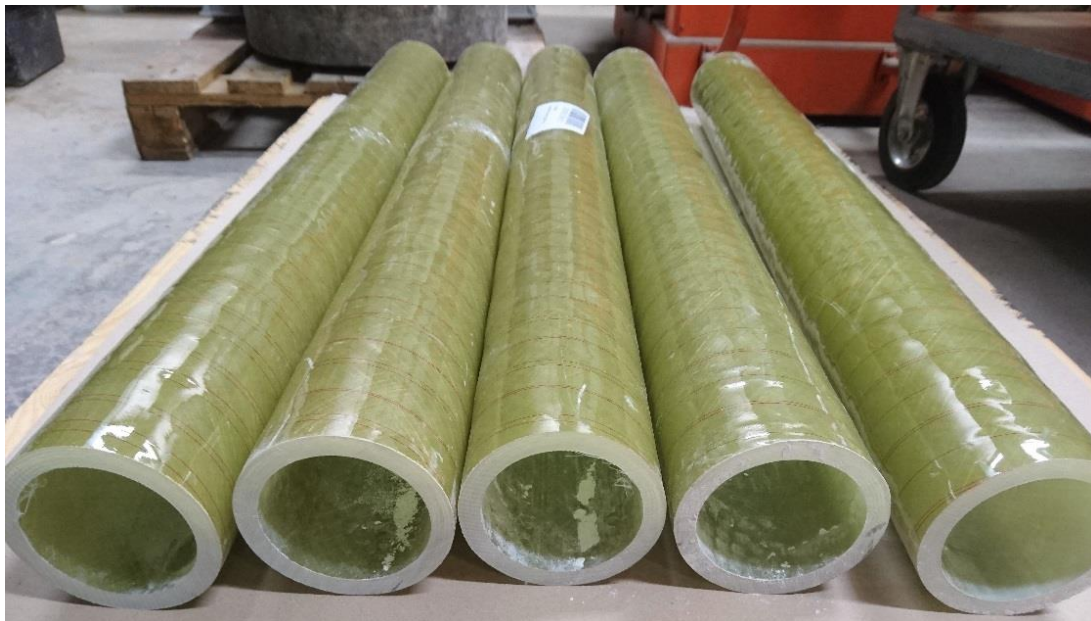
Figure 1. Decommissioned FRP insulation tubes from ABB Composites AB that were ground and used as filler in cementitious and polymer matrix composites.
