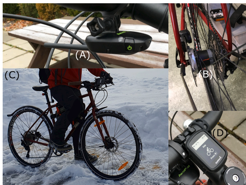
Fig. 2. Airspeed, air density, and road slope sensor (A) Pedaling power sensor (B) Instrumented bicycle under winter conditions (C) GPS tracking device (D).
