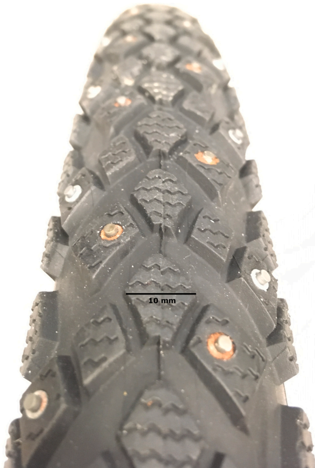
Fig. 3. Tread of the tire used in the experiments (Schwable Marathon Winter Plus).
