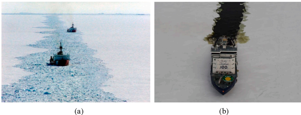
Fig. 6. Ice channels created by an icebreaker. (a) Brash ice channel (Credit: US Coast Guard) (b) Open-water ice channel (Credit: Aker Arctic).
