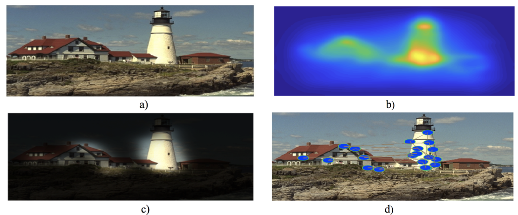
Figure 2. Example of a predicted scanpath of a given image: (a) Distorted image, (b) its saliency map from the GBVS method [78], (c) its highlight image and (d) the predicted scanpath.
