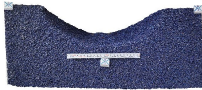
Figure 9. Dense point cloud of flushing cone for Test no. 3, Case study III
