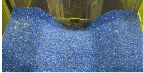
Figure 2. Flushing cone formed with PMMA.
