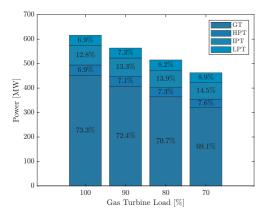
Fig. 3. Power distribution of the natural gas combined cycle with CCS at different gas turbine loads.
