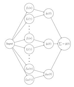
Fig. 2. Structure of a generic local model network.
