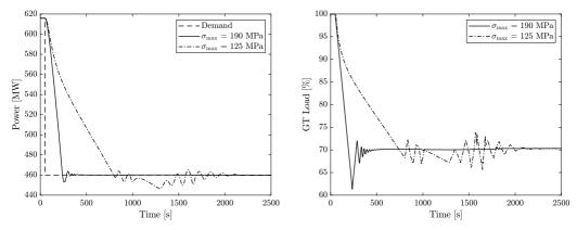
(a) Mechanical power generation with different stress constraints in the drum.
