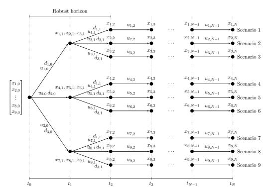
Figure 5.5: Schematic representation of a scenario-tree with  $M_{\rm r} = 3$  uncertainty realisations and a robust time horizon  $N_{\rm r} = 2$ .
