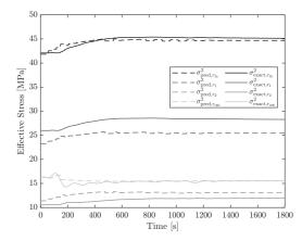
Fig. 16. Estimated and exact equivalent stress in the rotor at different radii.
