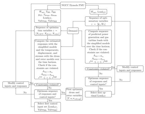
Fig. 6. Logic diagram of the MPC control strategy.
