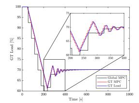
Fig. 8. Load profile of the gas turbine with MPC optimization steps.
