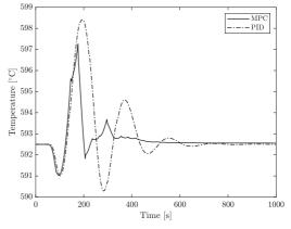
Fig. 12. Control of the reheat steam temperature.
