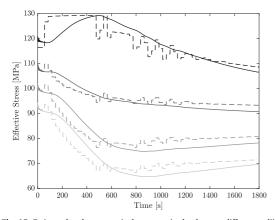
Fig. 15. Estimated and exact equivalent stress in the drum at different radii.
