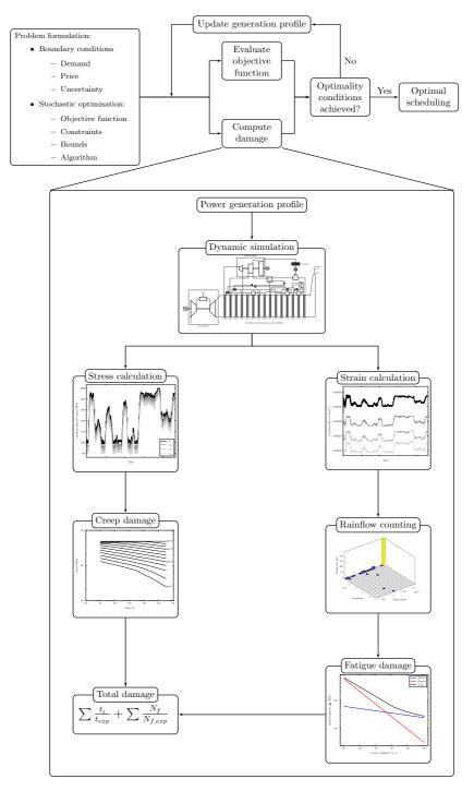
Figure 5.1: Method to optimally schedule the power generation profile of thermal power plants with lifetime enhancement under uncertainty.
