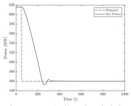
Fig. 7. Net power generation of the natural gas combined cycle.
