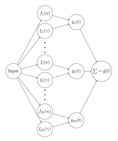
Figure 4.2: Structure of a local model network.
