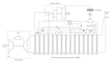
Fig. 2. Process model of the natural gas combined cycle. The nomenclature in the HRSG is as follows. E: Economiser, B: Boiler, S: Superheater, R: Reheater P: Pressure, L: Low, I: Intermediate, H: High.
