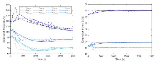
(a) Equivalent stress in the high pressure steam drum along three equidistant radii.
