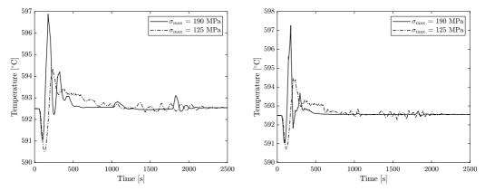
(a) Superheated steam temperature with different stress constraints in the drum.
