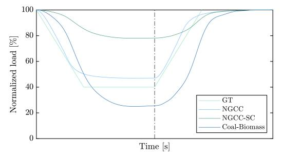
**Figure 3.1:** Generic dynamic behaviour of different thermal power plants of similar size. Maximum and minimum loads and power generation shares depend on power plant design. The vertical line indicates increasing load dynamic behaviour. The nomenclature is as follows. GT: gas turbine, NGCC: natural gas combined cycle, SC: steam cycle.
