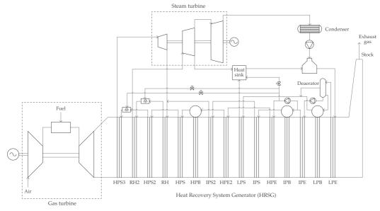
Fig. 1. Process model of the natural gas combined cycle. The nomenclature in the HRSG is as follows. E: Economizer, B: Boiler, S: Superheater, R: Reheater P: Presure, L: Low, I: Intermediate, H: High.
