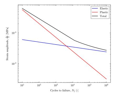
**Figure 5.4:** Diagram with experimental data to estimate the fatigue damage. The black line represents the maximum experimental number of cycles to failure given that a strain amplitude is a combination of elastic and plastic effects.
