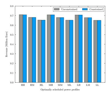
**Figure 5.9:** Revenue for the different scenarios considered in the stochastic optimisation with and without damage constraints. H, M and L indicate the high (105%), medium (100%) and low (95%) values of the power demand. A pair of letters defines two uncertainty realisations and hence the trajectory of each scenario.
