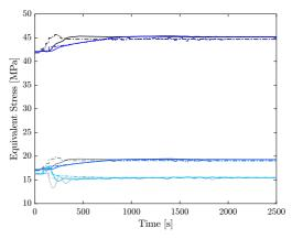
Fig. 8. Equivalent stress in the high pressure rotor disk along three equidistant radii.
