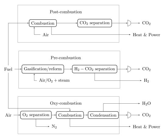
Figure 2.7: Schematic representation of CO<sub>2</sub> capture systems for power generation.
