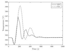
Fig. 11. Control of the superheat steam temperature.
