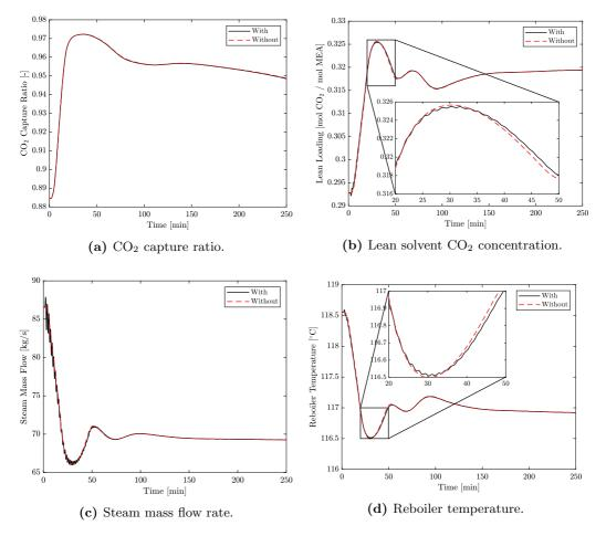
Figure 3.5: Dynamic behaviour of key process variables in the post-combustion capture plant during a gas turbine load change from 100% to 70% with and without fast dynamic fluctuations in the steam extraction valve.
