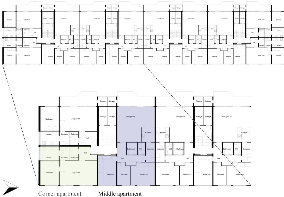
FIGURE 5.5. Floor plans of a typical apartment block with the two representative apartments marked in green (corner apartment) and blue (middle apartment).
