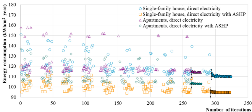
Figure 7. Minimization of the objective function in the simulation-based optimization (i.e., IDA ICE plus GenOpt).
