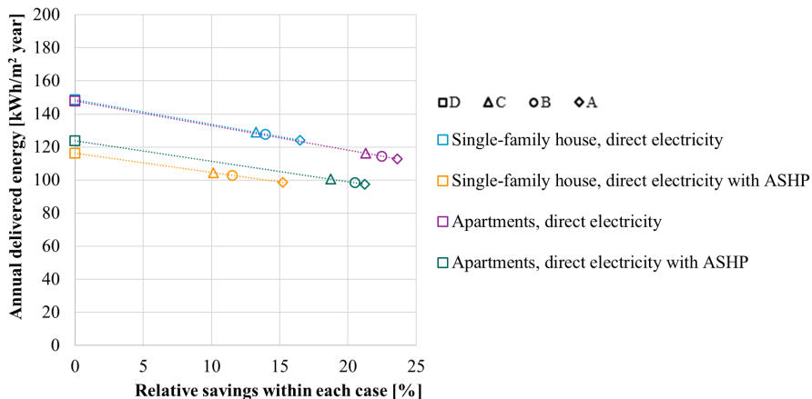
FIGURE 6.7. Impact of upgrading building automation control strategies on four different cases using control strategies and setpoints according to approach II.
