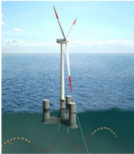
Figure 1 The OO-Star Wind Floater Semi 10MW concept [29]
