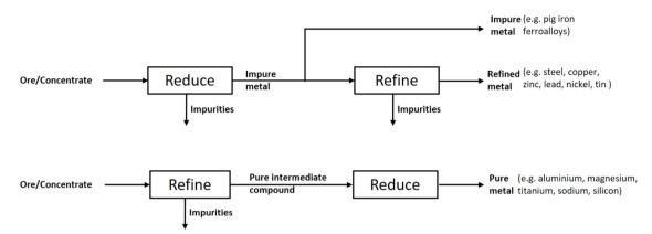
Fig. 4. Reduce and refine or the other way around. Adaption of Figure 8.4 pp. 158 in [4].
