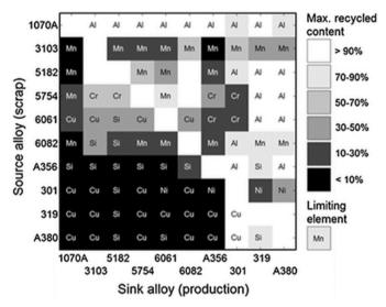
Fig. 8. Options and constraints for recycling of typical automotive aluminum alloys. Greyshades indicate the percentage of a source alloy (scrap) that could be used in production of a sink alloy. Limiting elements for recycling are indicated in each square [11].
