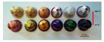
Fig. 18. Different coffee capsules before and after holding at 500 °C for 3 h [23].
