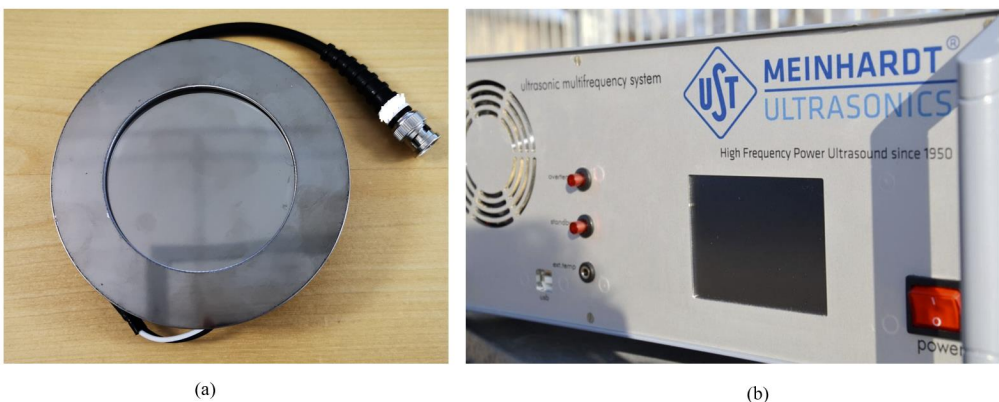
Figure 16. Honda 488 kHz plate transducer (a) and Meinhardt ultrasonic multifrequency system (b)
