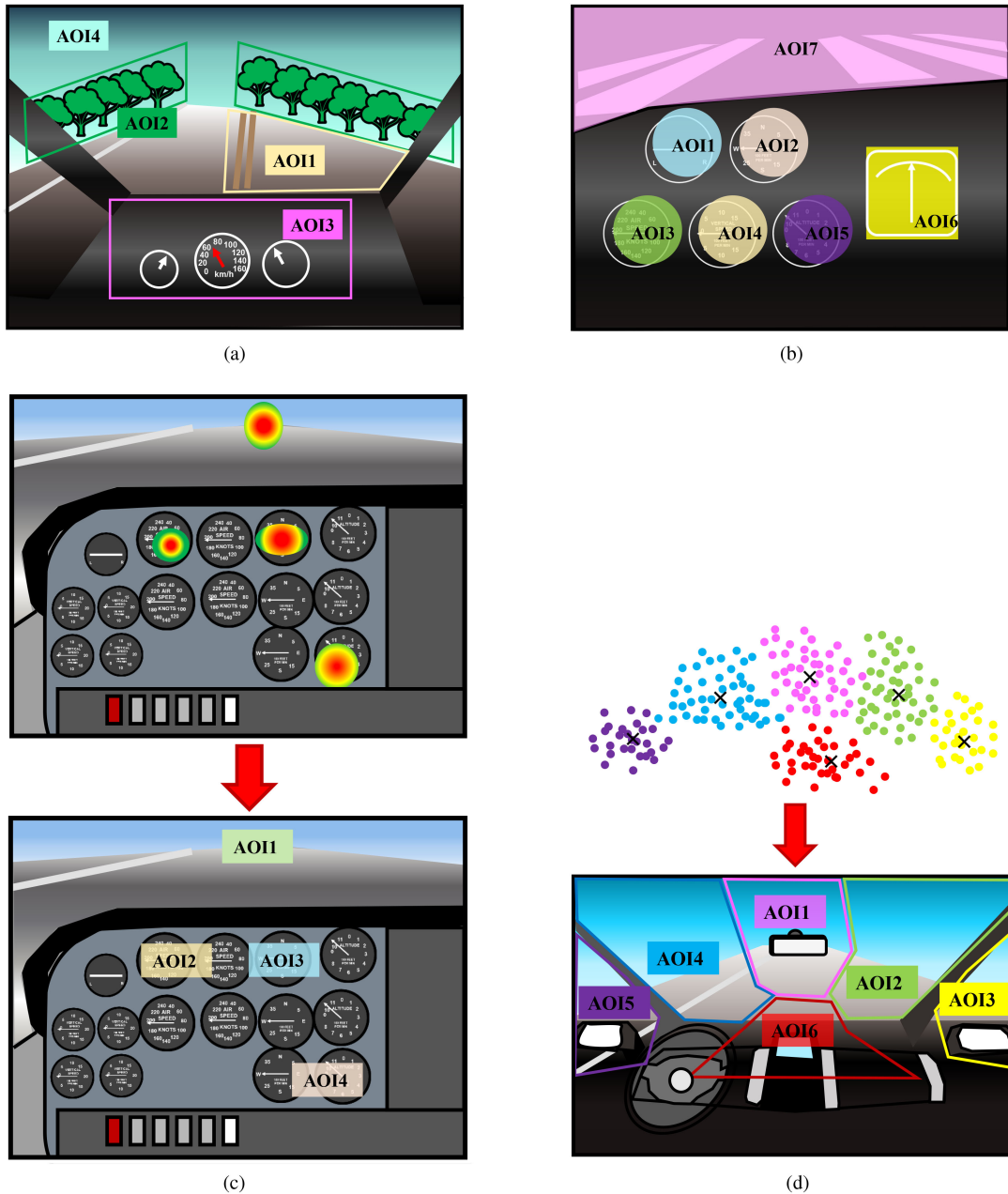
Fig. 4. Typical AOI setting definitions determined by (a) experts (adapted from [32]), (b) generation from stimulus (adapted from [68]), (c) attention map (adapted from [40]), and (d) clustering algorithm (adapted from [75]).
