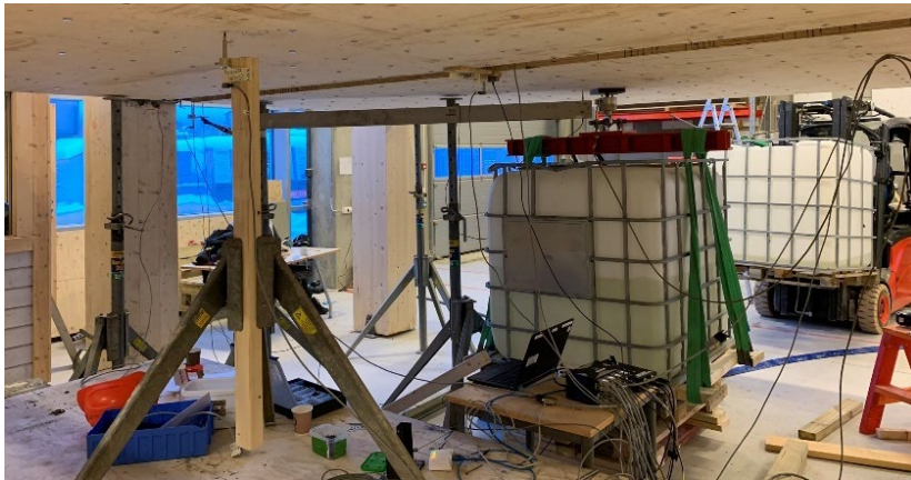
Fig. 10: Static load test situation image
