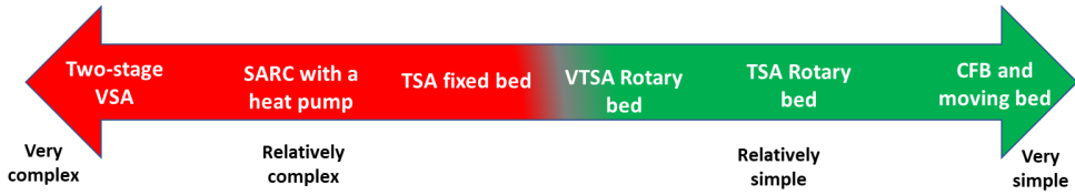
Figure 2-19: A simplistic illustration of the extent of complexity of the operating strategy of the different reactor configurations and operating mode.
