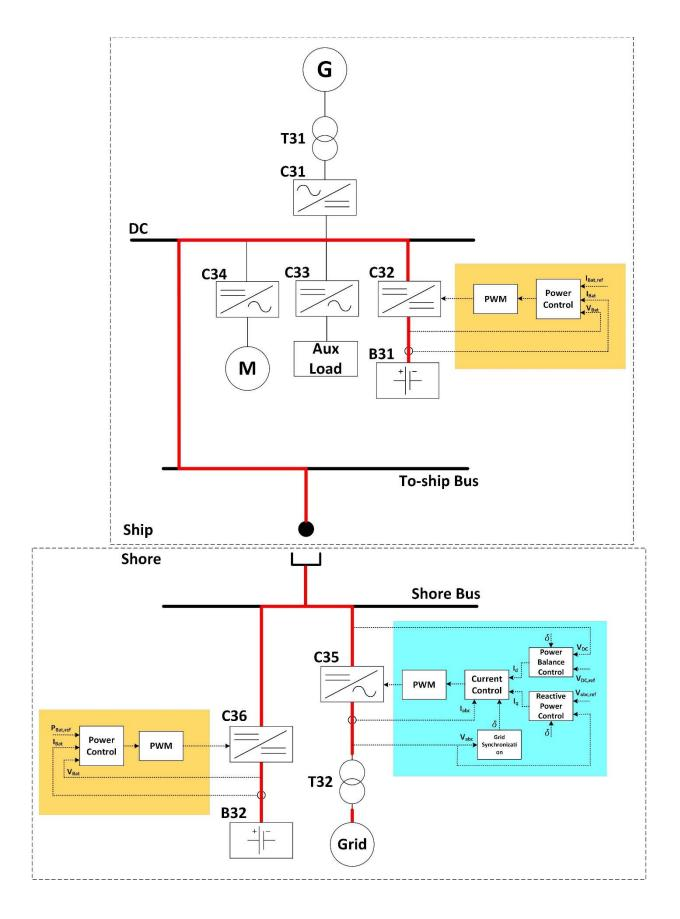
Figure 15. Converter control for charging path
