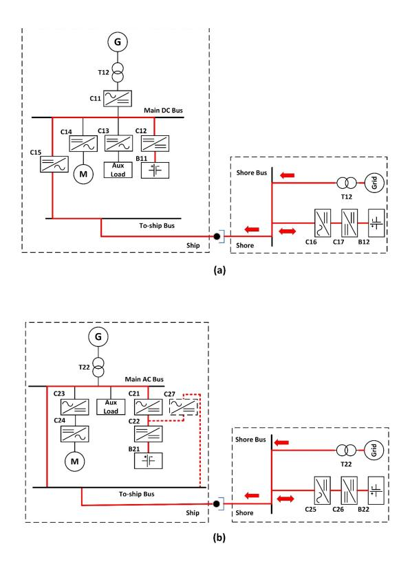
Figure 1: AC shore-to-ship charging for (a) a DC-microgrid-based and (b) an AC-microgrid-based propulsion system
