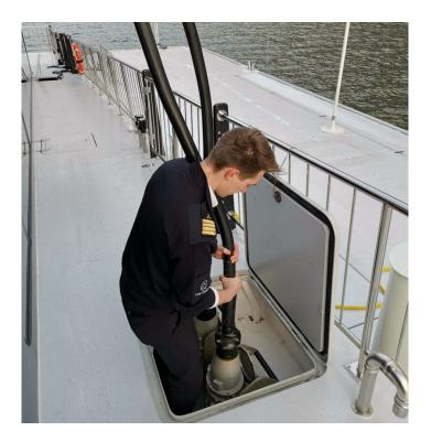
Figure 5: manual connection of two cables for charging the future of the fjords. Photo: Severin Synnevåg
