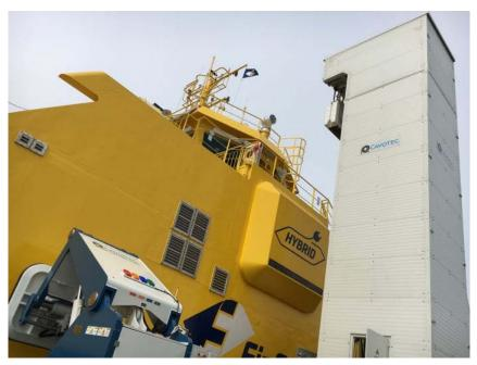
Figure 8: Cavotec APS tower used for charging MF Elektra. Photo: Cavotec
