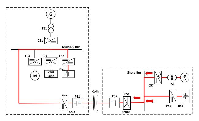
Figure 3: Inductive shore-to-ship charging for a DC-microgrid-based propulsion system
