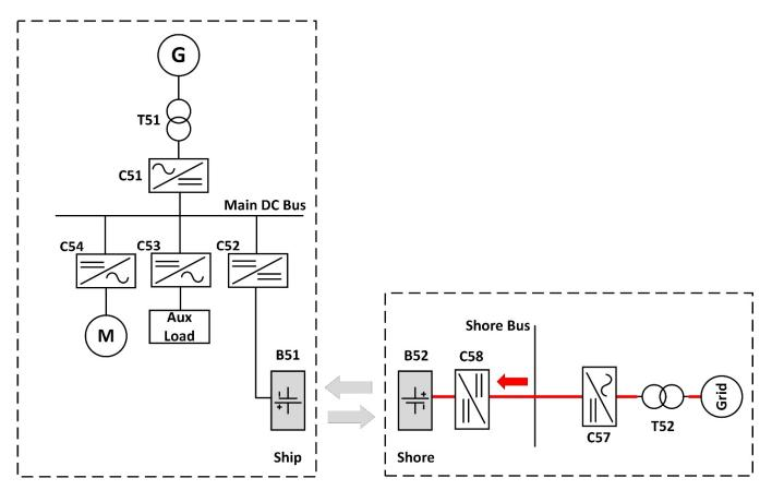
Figure 4: Battery swapping method
