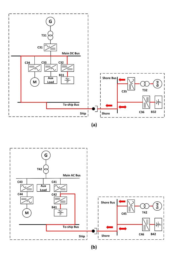
Figure 2: DC shore-to-ship charging for (a) a DC-microgrid-based and (b) an AC-microgrid-based propulsion system
