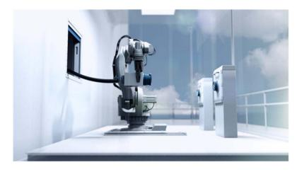
Figure 7: ABB IRB7600, an autonomous robotic arm used for charging MF Aurora and MF Tycho Brahe. Photo: ABB
