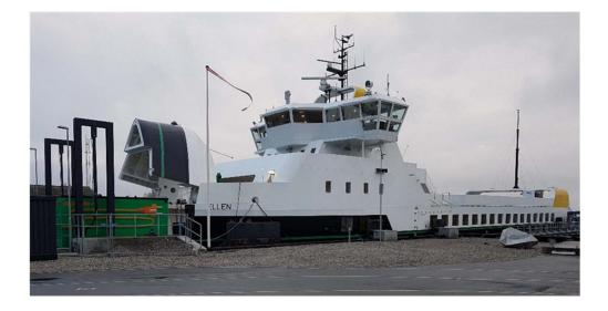
Figure 10: The Mobimar Nectors™ DC-based charging station for E-ferry Ellen, photo: Mobimar
