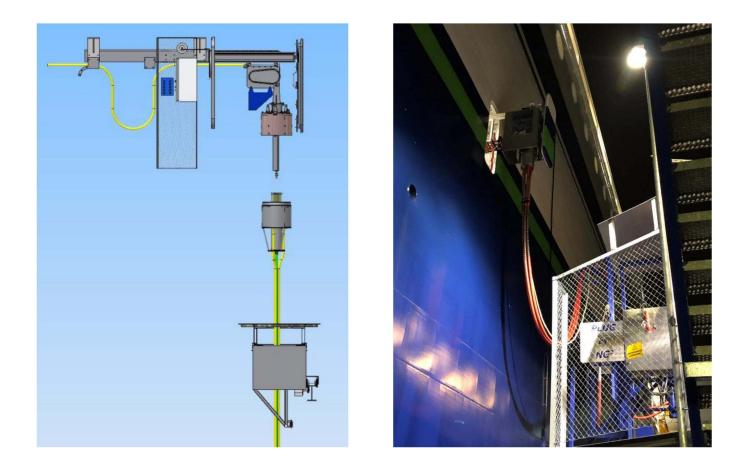
Figure 6: the typical PLUG structure and NG3 PLUG used for charging the Color Hybrid, respectively from right to left, photo: PLUG
