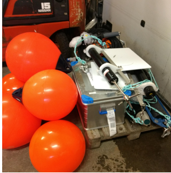
Figure 2.1: A stack of instrumentation used during the experimental work done for this thesis. The sensors were attached to the orange buoys using rope at different depths. To the right of the box on the pallet is one acoustic Doppler current profiler from Nortek and one from Aanderraa (ADCP/DCP). Ontop of the box is a Nortek Vector (ADV) with a "wing" attached to make it turn towards the current. Behind it is an Otopode with its sensing head protected by bubble-wrap.
