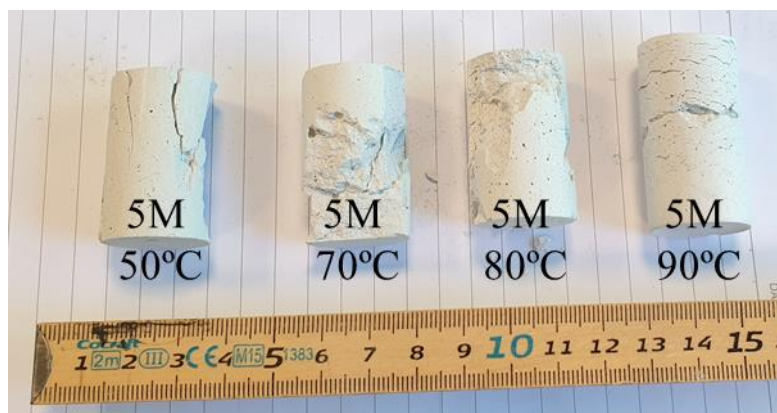
Figure 5 – Colour of samples after compressive strength testing and storage in plastic bags for several months
