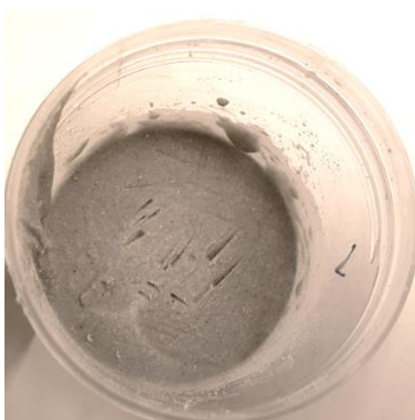
Figure 2 – Representative example (5a) of visual appearance of a hardened PA-An paste after 14 days, with spatula marks in the surface
