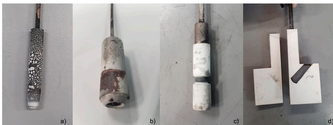
**Figure 12.** Pictures of the anodes after the experiment: (a) rod anode, (b) horizontal anode, (c) vertical anode and (d) inverted horizontal anode (cross-sectioned).
