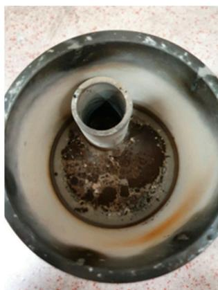
**Figure 16.** Image of the surface of the frozen bath in the silicon nitride crucible at room temperature after the experiment with the rod anode and inverted horizontal anode.
