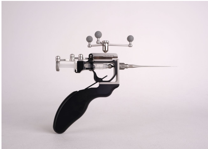
Fig. 2.—The MultiGuide, a novel injection device to perform surgical navigation-assisted procedures.
