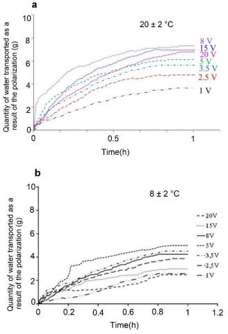
**Figure 5**: The quantity of transported water over time as a function of applied voltage at ambient temperature of: a)  $20 \pm 2 \degree C$  [40], and b)  $8 \pm 2 \degree C$  [39].
