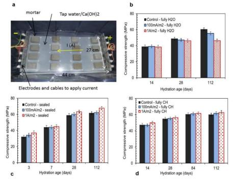
Figure 4: a) Experimental set-up for DC curing of samples submerged in water and Ca(OH)<sub>2</sub> solution [50]. Compressive strength as a function of curing time for mortar samples under current flow conditions: b) submerged in H<sub>2</sub>O; c) sealed condition; d) submerged in Ca(OH)<sub>2</sub> solution [49].
