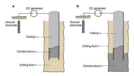
Fig. 8: Schematic view of the well showing the apparatus for: a) cleaning the casing from the drilling mud; b) increasing the bonding of cement to casing by DC field application, after [80].
