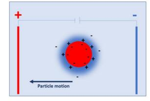
Figure 1: Electrophoretic movement of a charged particle in an aqueous solution with the application of electric field, after [32].
