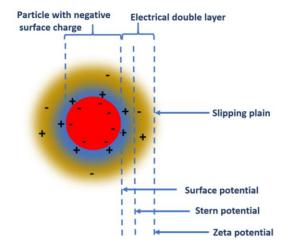
**Figure 2**: Schematic representation of the double layer surrounding a charged particle, after [22]. The zeta potential, the main parameter determining the electrokinetic behavior of the particle, is the potential at the slipping plane.
