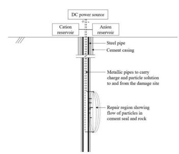
Figure 9: Proposed method applied to a wellbore [85].
