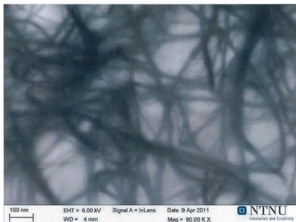
**Figure 58: Nano scale treads in pale blue condensate at very high magnification. The diameter of the treads is varying in the range 10 - 30nm. [54]**
