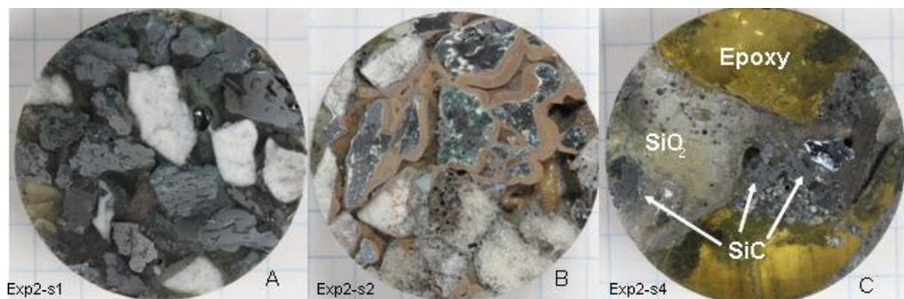
**Figure 52: a) Charge before condensation (1450°C); b) Brown condensate formation at 1600°C; c) Molten quartz surrounding SiC particle (1760°C). [68].**
