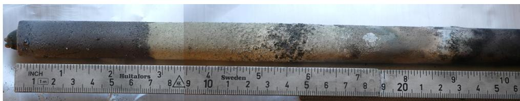
**Figure 239: Graphite tube protecting the thermocouple in the large-scale setup, Experiment IF3a.**
