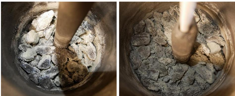
**Figure 167:** Left: Stoking point  $Y = 21$  cm,  $T=1420^\circ\text{C}$ , Exp IF75-7a. Right: Brown condensates at  $Y = 18$  cm,  $T = 1580^\circ\text{C}$  for experiment IF75-7a.
