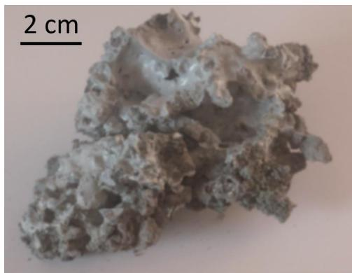
Figure 26: Stoking crust containing molten quartz and condensate, extracted from a FeSi75 furnace [56].
