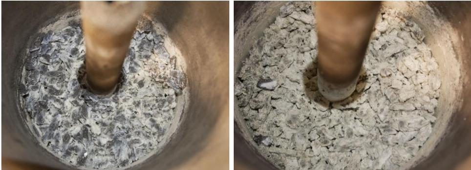
**Figure 166:** Excavation of the crucible at  $Y = 18$  cm,  $T = 1485^\circ\text{C}$ . SiC charge before (left) and after poking (right), experiment IF2a.
