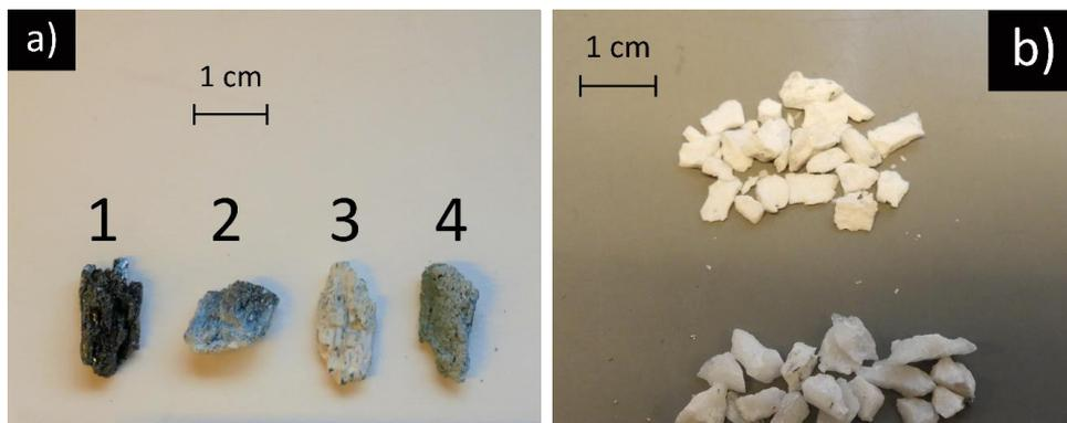
Figure 94: Samples from Experiment IF10,  $T = 1370\text{-}1650^\circ\text{C}$ . a) 1) SiC particle without condensate; 2) SiC covered in white and blue condensate; 3) SiC covered in white condensate. 4) SiC covered in grey condensate. B) Top: Quartz A covered in white condensate; Bottom: Quartz A without deposition of condensate.
