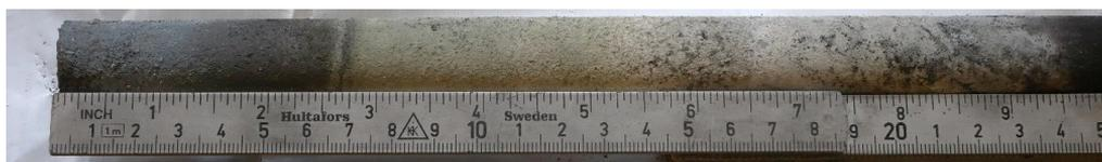
**Figure 238: Graphite tube protecting the thermocouple in the large-scale setup, Experiment IF2a.**
