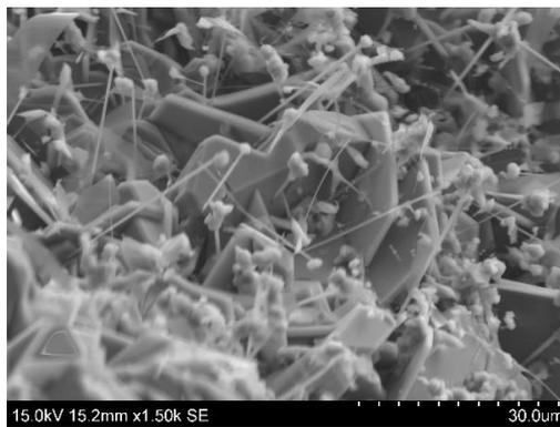
**Figure 230: Droplet SiC whiskers from experiment R6a.**
