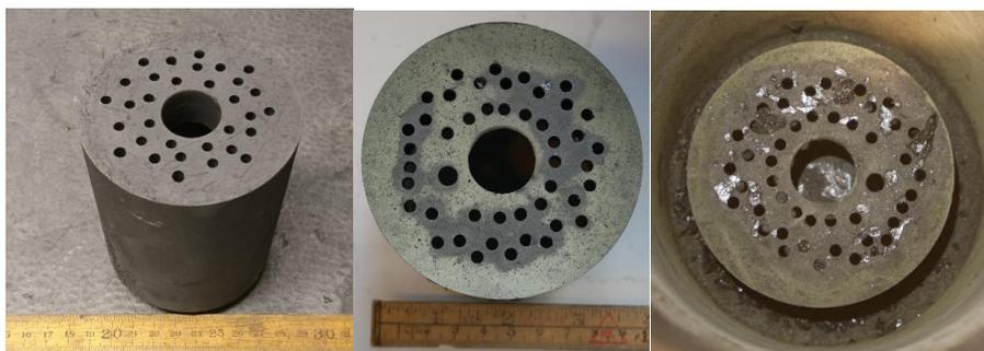
**Figure 227:** Left: Gas production chamber before Exp. 3a; Center: Top view of green layer on gas production chamber, Exp. 1a; Right: Top view of green and grey layer on gas production chamber, Exp. IF2a.
