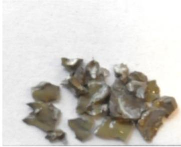
**Figure 202: Tones of dark and light brown in condensate sample, T = 1580-1706°C, Experiment R4c**
