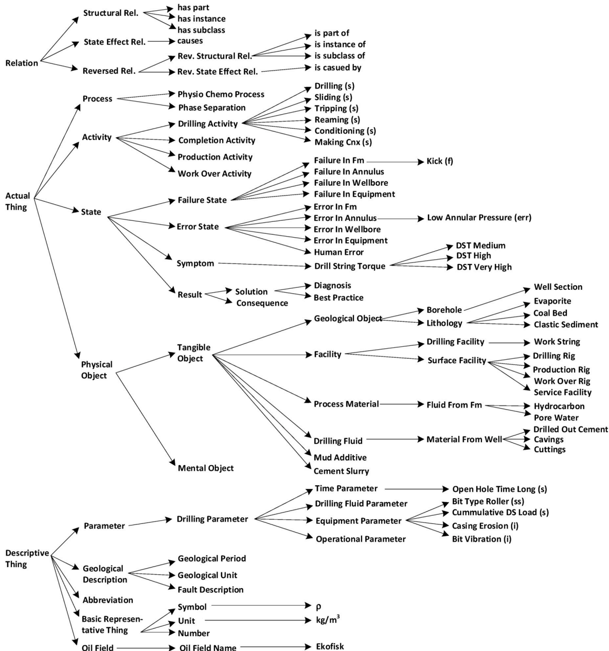
Fig. 5. Expanded Structural Knowledge model of the Drilling Process, including specific examples at lower sub class levels.
