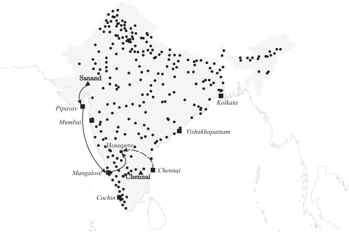
Fig. 3. Map of India with two production facilities, seven ports along the Indian coastline and 261 customer locations.
