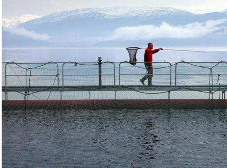
Figure 2.1: Floater of a steel type fish farm. The floater appears as a semi-submerged horizontal cylinder. The floater has a circular cross-section with diameter 1m. A walkway is mounted to the floater.
