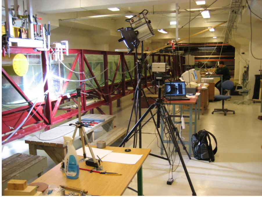
Figure 6.2: From the wave laboratory. The circular model, seen to the far left, is mounted to the rig. The photo is taken towards the wavemaker side of the flume.
