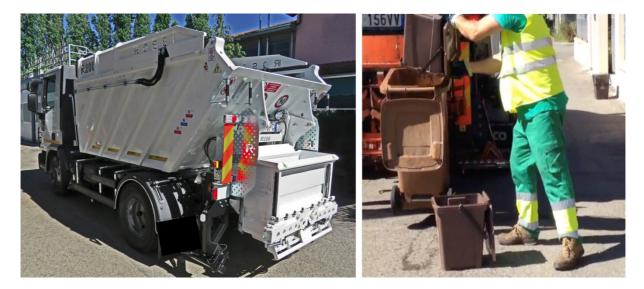
Fig. 1. On the left, the collection vehicle. On the right, two-handed tip of the plastic bin intothe truck container on the back of a collection vehicle.
