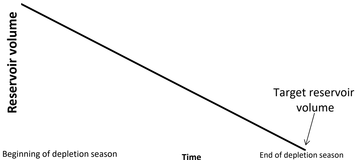
Figure 16: Tapered reservoir volume trajectory in the depletion season. Tapered from full reservoir volume to an end of the depletion season target reservoir volume.
