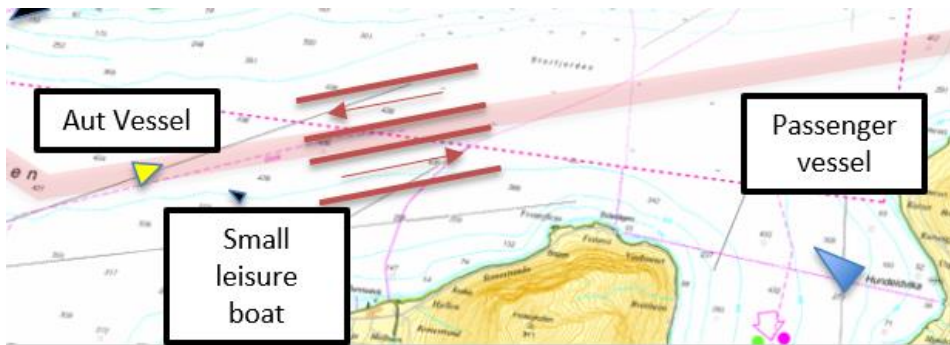
Figure 8: The automated vessel might experience conflict situation with vessels under VTS control and vessels not controlled by the VTS
