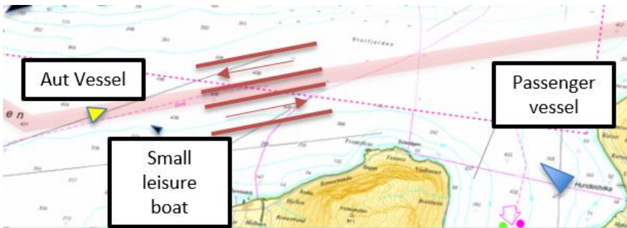
Figure 21: The automated vessel might experience conflict situation with vessels under VTS control and vessels not controlled by the VTS
