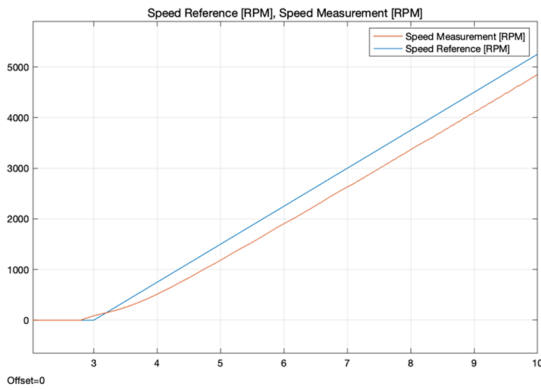
Fig. 11. Motor speed simulation result
