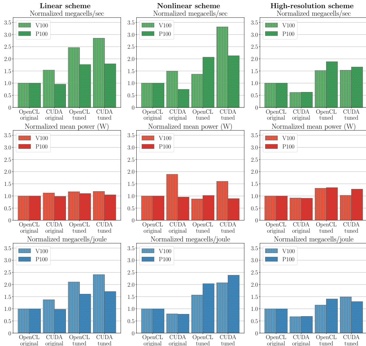
Figure 8. Comparison of original, ported, and optimized codes measured in megacells per second (top row), mean power usage (mid row), and megacells per joule (bottom row), normalized with respect to the original OpenCL implementation, for the Tesla P100 and V100 GPUs. The power is measured through nvidia-smi and represents the power consumed by the GPU only. On the V100, there are only minor differences in mean power consumption between different versions of the linear and high-resolution scheme, but CUDA uses more power than OpenCL for the nonlinear scheme. CUDA is, however, more power-efficient than OpenCL for all three tuned schemes on this GPU. On the P100, the mean power consumption is equal for all versions of the linear and nonlinear schemes, which means that power efficiency becomes equivalent to computational efficiency. For the high-resolution scheme, we see that the mean power consumption increases for the tuned codes, but the computational performance increases more, meaning that the power efficiency is still improved by 30%–40%.
