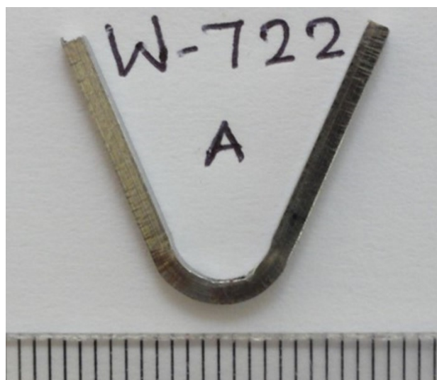
Figure 12. Typical face bent specimen.
