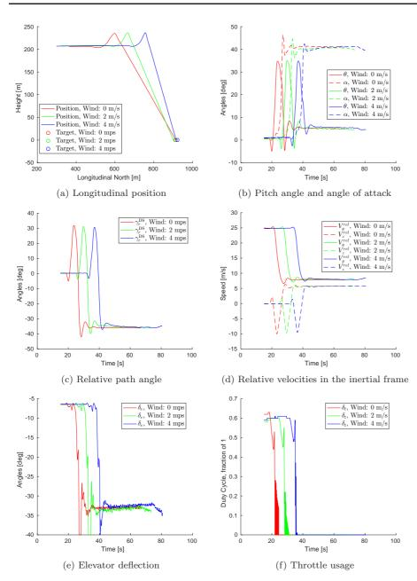
Fig. 6: Estimated variables of the UAV while controlled by an NMPC from cruise to deep-stall, for steady wind equal to 0 m/s, 2 m/s and 4 m/s, with a light turbulence.
