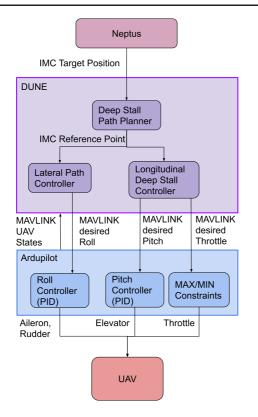
Fig. 4: Control system structure for deep-stall manoeuvre.
