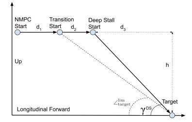
Fig. 3: The longitudinal reference path for the deep-stall landing
