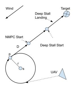
Fig. 1: The lateral path for the landing. Before longitudinal NMPC guidance is initiated, the UAV is guided with line-of-sight-based lateral and longitudinal controllers.
