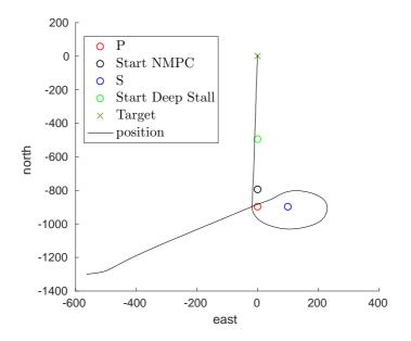
Fig. 5: The lateral flight path of the UAV before and in the deep-stall, with 4 m/s wind.
