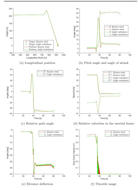
Fig. 7: Estimated variables of the UAV while controlled by an NMPC from cruise to deep-stall, with 4 m/s wind and no or light turbulences.
