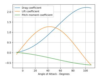
Fig. 2: The drag coefficient, the lift coefficient and the pitch moment coefficient of the UAV model used in this paper, with respect to the angle of attack.
