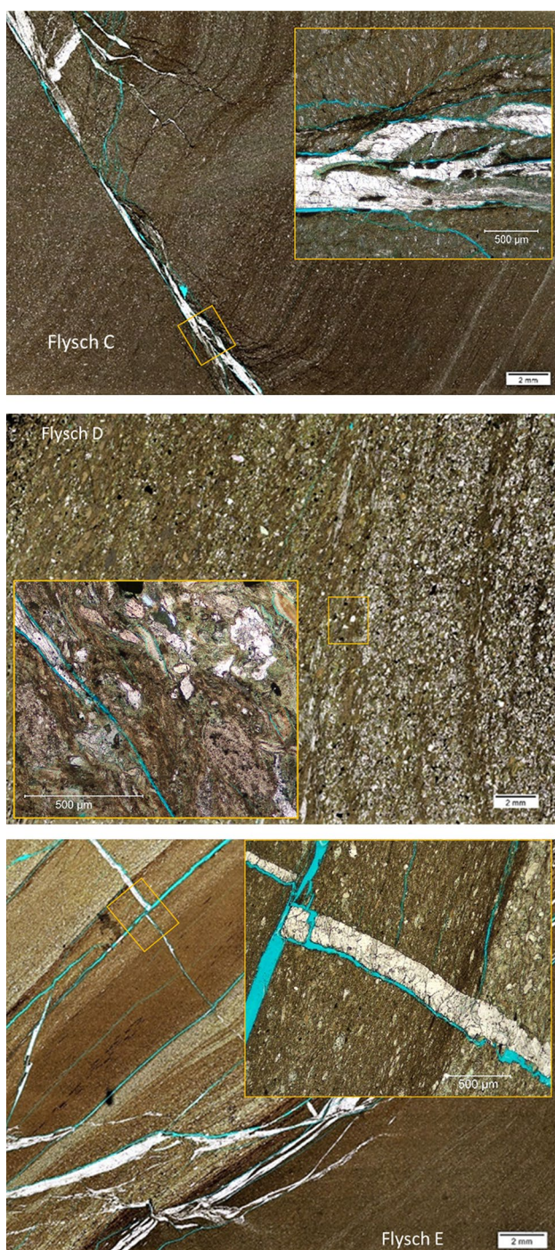
Fig. 3 Thin-section scans of Flysch C–E, including magnifications of fracture details (yellow boxes) (color figure online)
