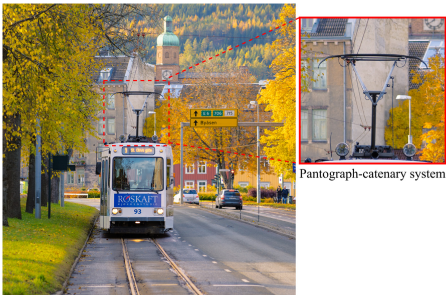
Fig. 28. Trams with the pantograph-catenary system. Photo: Tengjiao Jiang/NTNU.
