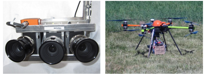
Fig. 2. Left: The three cameras with partially overlapping FOV across track. Right: The sensor payload mounted on a UAV.
