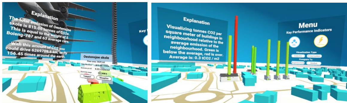
Figure 2. Snapshot in ZEN View of the Sluppen area using VR to visualise emissions of buildings
