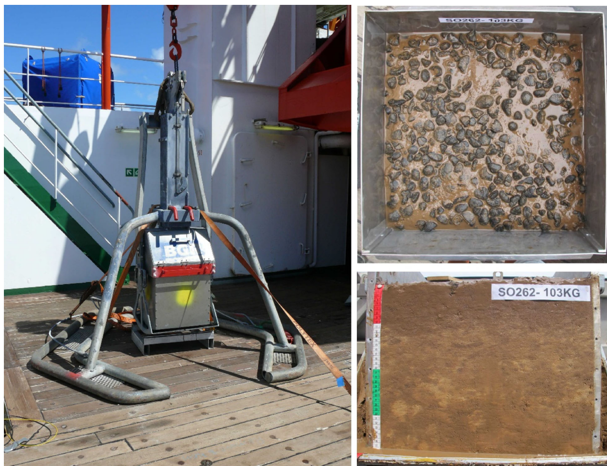
Figure 2. Box corer used for sampling of seafloor sediments and nodules (left panel) as well as surface (upper right) and downcore profile (lower right) of the sediment block sampled.
