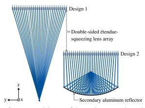
**Fig. 4.** Ray-traced drawing of the two design examples. Only a subset of the lens pairs is drawn and traced, to reduce clutter in the drawing. In reality, the lens pairs are tessellated to fill the entire front and back surfaces of the lens array, as shown in Fig. 3.
