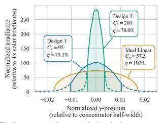
**Fig. 5.** Intensity profile across the focal line for the two concentrators, under 1 sun AM1.5D illumination with a  $\pm 1^{\circ}$  top-hat angular distribution. The solid lines represent the intensity within the selected geometric concentration ratios. The non-uniform intensity profile of the ideal linear concentrator is caused by the circular  $\pm 1^{\circ}$  angular distribution of the illumination, as further discussed in Supplement 1.
