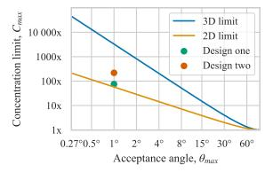
**Fig. 1.** Concentration limits versus acceptance angle, as given by Eqs. (1) and (2), shown on a log–log scale. The line-focus concentrators demonstrated in this work, represented by the symbols green and red circle, have concentration ratios beyond the 2D concentration limit.
