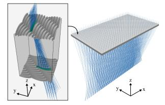
**Fig. 3.** Solar concentrator utilizing étendue squeezing, consisting of an array of tessellated étendue-squeezing lens pairs. Each lens pair squeezes the beam in the x direction and expands it in the y direction, while redirecting the sunlight towards the common focal line. The cutout shows one such lens pair highlighted in green, and demonstrates how the lens pairs are tessellated into a complete double-sided lens array.
