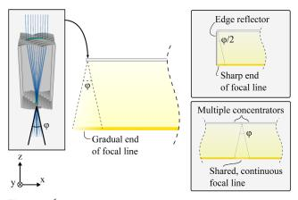
**Fig. 7.** Étendue-squeezing lens pairs increase the angular extent of the light along the x direction, which introduces a softening at the ends of the focal line. This effect can be circumvented by creating a long assembly of concentrators sharing the same focal line, or by using an edge reflector.
