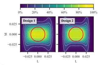
**Fig. 6.** Optical efficiency of the concentrators as a function of incidence angle, shown as contour plots in direction cosine space. L and M are direction cosines along the x and y axes, respectively. The concentrators are optimized for maximum efficiency under a  $\pm 1^{\circ}$  top-hat angular distribution, which is illustrated by the red circles.
