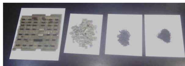
Fig. 2. The process steps to obtain the metal-powder from PCB.
