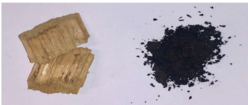
Fig. 2. Pre-treatment of lignocellulosic materials can change the structure of lignocellulose significantly. For example, steam explosion treatment of birchwood. Left: chips of around 30 mm prior to steam explosion; right: the dark and sticky birchwood with a less obvious fibre structure after steam explosion.
